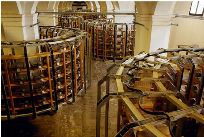
Fig. 1. RI studies on ELFEMF: exposure system. The exposure system was based on independent devices, each one serving at least 500 rats. The toroidal shaped device guaranteed the absence of interference between the structures. A wooden support structure for rat cages was mounted inside the toroidal magnet. Note that the toroidal structures were all located in a unique room of more than 900 m 2 , in order to ensure a homogeneous conduct of the experiments.
